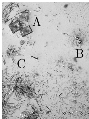
Figure 20. Crystalline product of the reaction between \text{ThO}_2 and sulfuric acid. The larger plates (A) are \text{Th}(\text{SO}_4)_2 , whereas \text{Th}_4(\text{HSO}_4)_2(\text{SO}_4)_7 forms small polyhedral crystals (B). The main product is \text{Th}(\text{HSO}_4)_2(\text{SO}_4) , which crystallises in the form of small hexagonal needles (C).
